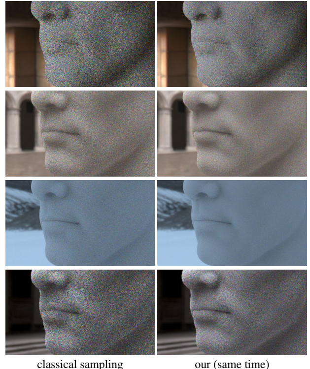
Figure 3: Despite the fact that the importance function driving the sampling assumes uniform hemispherical illumination (that is, all directions upon escaping from the medium have the same importance), the modified path sampling lowers variance even when the illumination is nonuniform. The images rendered with classical sampling use 100 samples/pixel while in our results we trace about 50% more samples/pixel in the same time. While the speedup is a profitable side-effect, most of the variance reduction is due to the sampling pdfs closely approximating the zero-variance sampling scheme. As in Fig. 1, the subsurface medium has a single-scattering albedo of 0.943 for all wavelengths and index-matched smooth boundaries. The individual rows show results for different environment maps. The first two rows show the same images as in the abstract.
