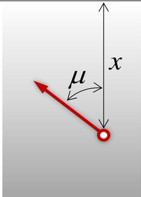
$$\phi(x, \mu) = \int_{-1}^1 \underbrace{\phi(v, \mu) e^{-x/v}}_{\text{transient terms}} dv + \underbrace{\phi_0(v_0, \mu) e^{-x/v_0}}_{\text{asymptotic term}}$$
