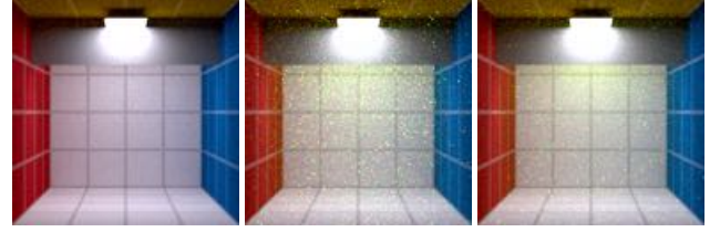
(a) Standard exponential tracking (b) Exponential tracking using \max(\hat{\sigma}_t, \hat{\sigma}_s) (c) The proposed fluorescence-aware tracking.
