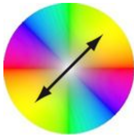
Figure 5: Colour coding of the linear polarisation false colour scheme proposed for use in visualisation 3 – the oscillation plane visualisation seen in figure 6. Linearly polarised light with the indicated oscillation plane would e.g. be encoded as yellow. In figure 6, the fringe of the sphere, which in its entire circumference contains linearly polarised light of all orientations, is a good example of what this looks like when used in an image.
