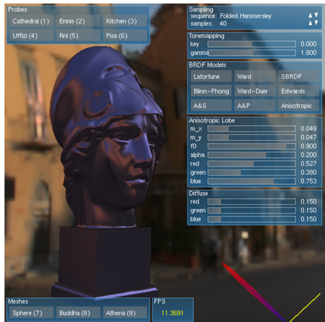
Figure 15: Material design can be done with analytical BRDF models on the fly. This is true for our proposed Anisotropic model as well.
