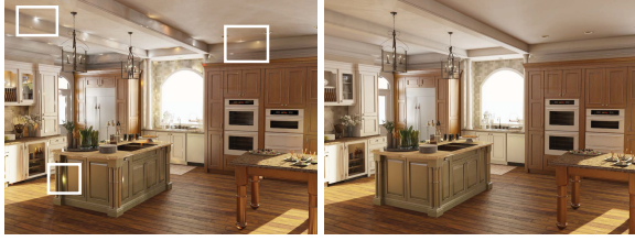
Figure 9: When not accounted for, the singularity in the geometry term produces high intensity splotches, which degrade the rendering quality (left). Several techniques address this problem producing images that do not suffer from these artifacts (right). Images courtesy of Edgar Velázquez-Armendáriz.
