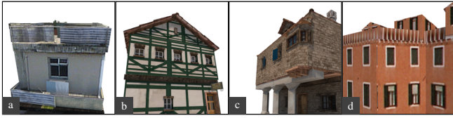
Figure 11: Computer generated images with implausible structures. (a) Balcony and roof without any access points ( a = 0.87 ); (b) Window placed in a support pillar, door too close to edge ( a = 0.96 ); (c) Wooden balcony support inside stone/concrete support ( a = 1.0 ) (d) Deformed roof structure and incorrectly applied texture ( a = 1.0 ).
