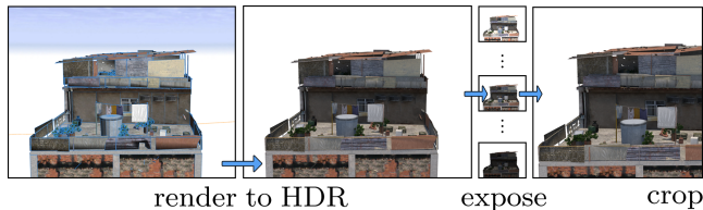
Figure 5: Computer generated image preparation workflow. A 3D model is rendered to an HDR file with full global illumination, the exposure is manually adjusted, and the image is cropped.
