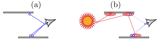
Fig. 22: Stochastic progressive photon mapping (SPPM) [35] works in two passes: (a) First, it generates a set of measurement points (blue) from the camera. (b) Second, a set of photon paths (red) from the light sources is generated and the image is computed by splatting photons (vertices of photon paths) onto nearby measurement points (red ellipse). This corresponds to performing density estimation over photons at each measurement point. The generation of measurement points and photon paths is iteratively repeated and the image estimates from each iteration are averaged. To ensure consistency of the method the density estimation radius is shrunk in each iteration.
