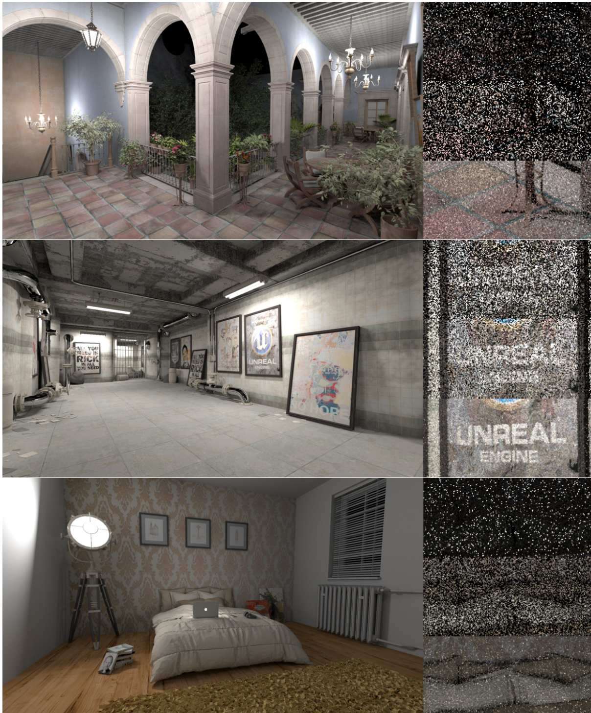
Figure 9: Algorithm comparison for different scenes. The zoomed areas have been rendered with 2 paths of length 3 per pixel and 4 shadow rays at each bounce. For each scene there are three zoomed areas. Top: Uniformly selecting one light source out of many. Middle: A light hierarchy. Bottom: Visibility-guided importance sampling. Unreal Engine demo by Epic Games.
