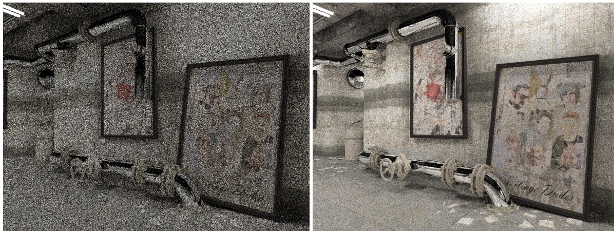
Figure 7: Comparison. Left: Uniform sampling. Right: The effect of resampling importance sampling: First, 8 samples are generated from a uniform distribution across the light sources. Then a cumulative distribution function (CDF) is determined using the unoccluded contribution of each of the initial samples. The actual shadow rays to be shot are determined by resampling the CDF. Unreal Engine demo by Epic Games.
