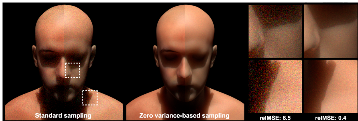
Figure 17: Path tracing of an optically dense medium (30 minutes), showing both a complete ‘beauty’ render ( S+V ), and a render with only volumetric transport ( V ). Building on an approximate adjoint solution of the incident and in-scattered radiance, our zero variance-based path construction forms near-optimal decisions for guided collision distance sampling, directional sampling, Russian roulette and path splitting. As such, our sampling methodology leads to significantly faster convergence compared to an unguided path tracer with standard transmittance-based collision and phase function sampling.
