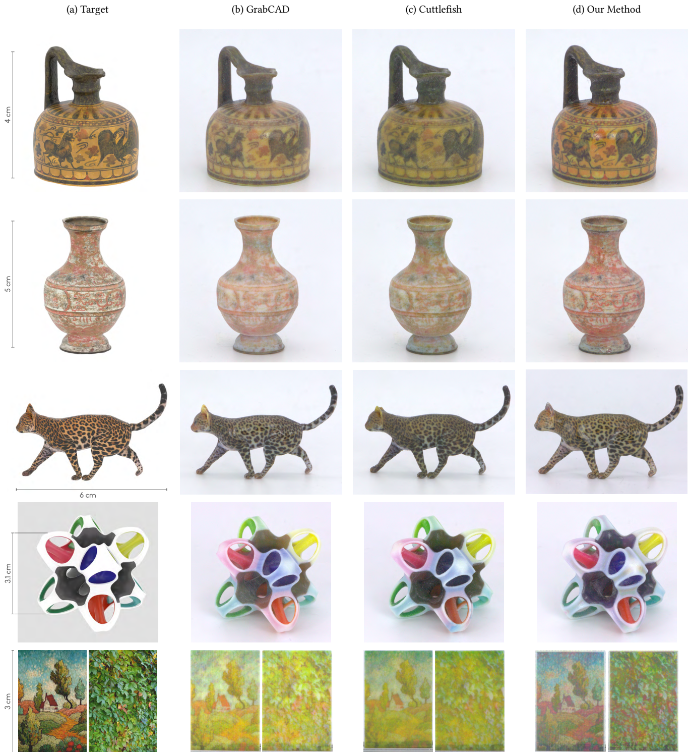
Fig. 14. Comparison of photographed printouts to the rendered (a) target models: (b) GrabCAD is the default printer software, (c) Cuttlefish is based on [Brunton et al. 2015], and (d) Our scattering- and crosstalk-compensated solution. The last model is a thin planar slab of 0.5 mm thickness with two different textures on its front and back sides.
