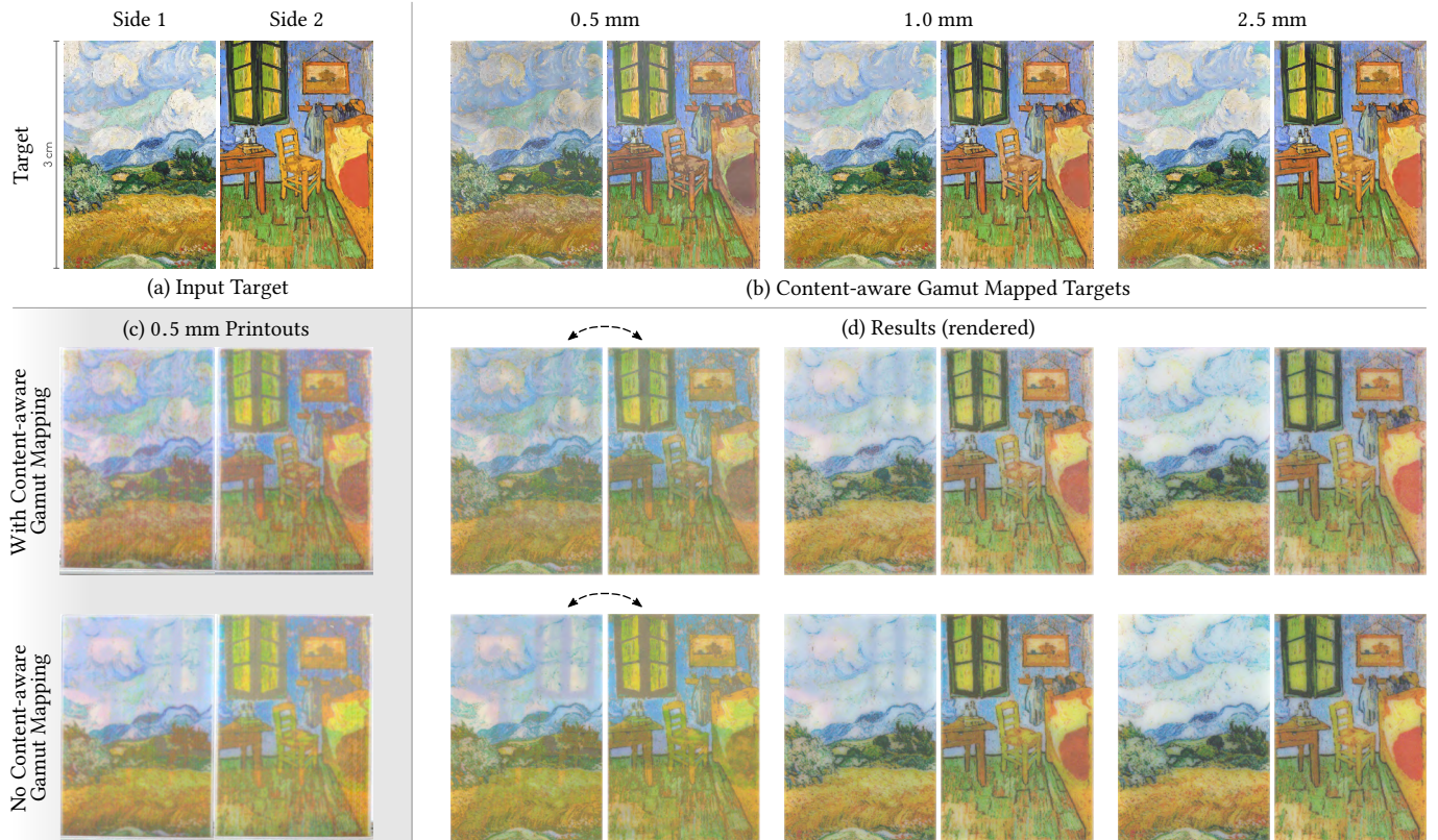
Fig. 12. Result of the content-aware gamut mapping demonstrated on planar slabs of different thicknesses (0.5, 1.0, 2.5 mm) with two images as target. (b) demonstrates the gamut-mapped target specification. The images on the gray background (c) are photographs of printouts as opposed to the rendered solutions in (d). Note the reduced cross-talk (i.e. the window under the arrow) and the reproduction of details and colors for the thinner cases.
