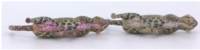
Fig. 17. Color shifts on the abdomen and blackening on the paws of a 2.5D remapped printout (left) compared to a native 3D printout (right). Similar setup as in Figure 16.
