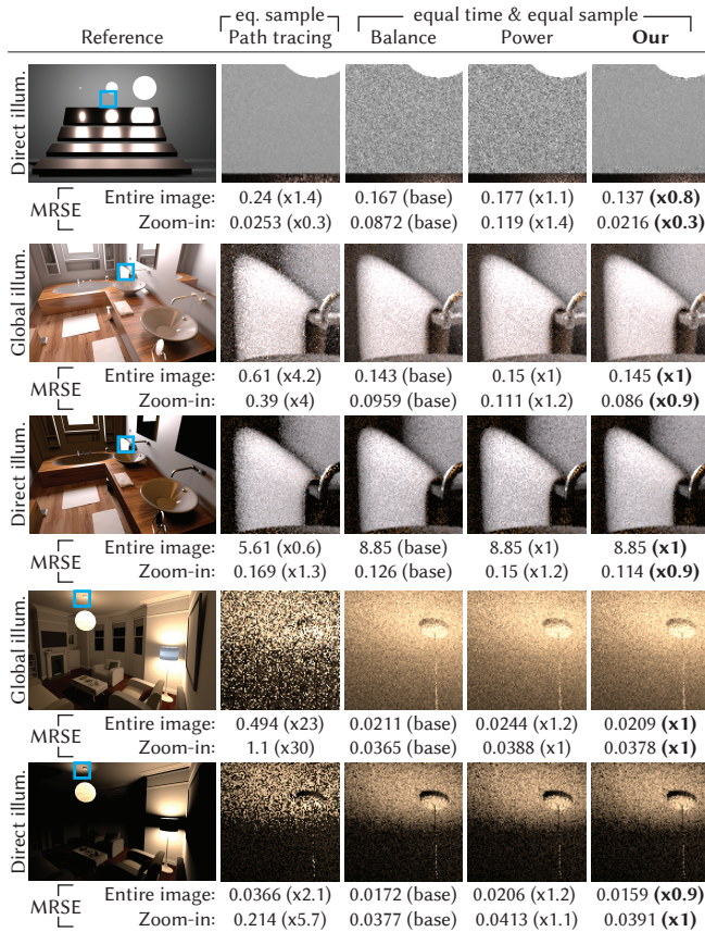
Fig. 4. Equal-time (and equal-sample) comparisons of BPT using three different MIS heuristics. Our heuristic improves low-variance cases while, in contrast to the power heuristic, never being significantly worse than the balance heuristic overall.
