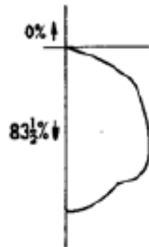
Porcelain-enameled ventilated standard dome with incandescent lamp
