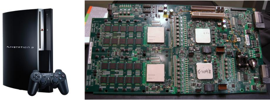
Figure 2.2: Images of Cell/B.E. based machines. Sony's Play Station 3, on the left (image taken from [www.boygeniusreport.com](http://www.boygeniusreport.com)), IBM Cell Blade board, on the right (image taken from [www.ps3tester.com](http://www.ps3tester.com))
