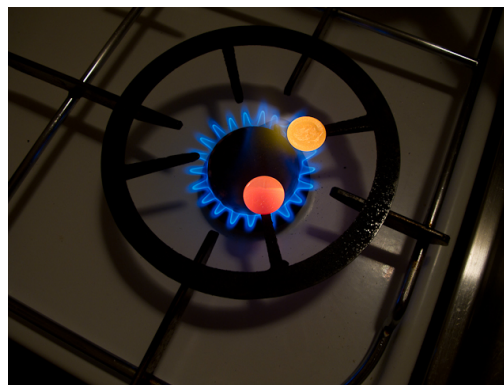
Figure 1: A photograph of two coins heated to approximately equal temperatures on a gas stove. At room temperature, the coin that glows red is silvery in appearance (nickel-plated steel), while the coin that glows yellow-orange is made of gold. Note the considerable hue difference.
