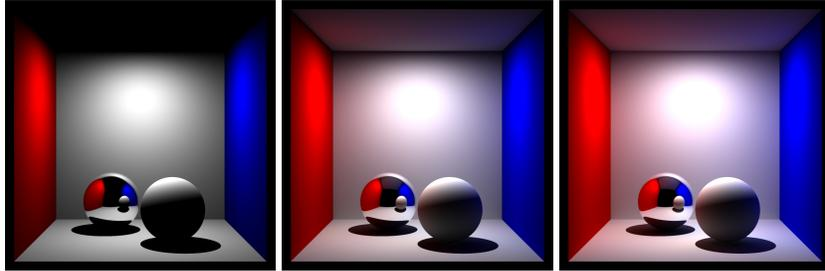
**Figure 12:** Cornell box with spheres: direct illumination, 1 bounce, and 2 bounces.
