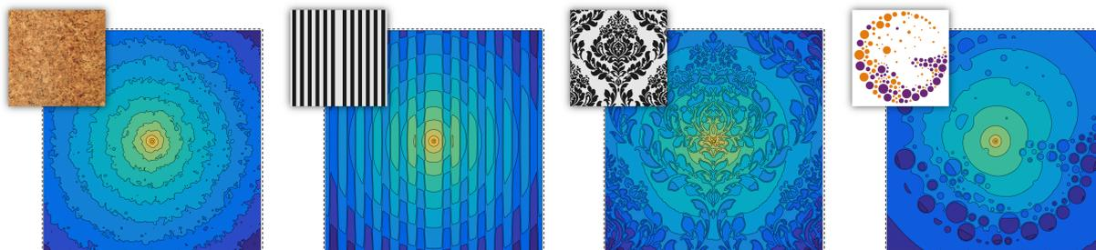
**Figure 1:** Predictions of the spatially varying sub-surface scattering kernels (false-color logarithmic maps) for heterogeneous materials (defined by 2.5D scattering albedo textures shown in the respective thumbnails). The proposed framework consists of two key steps: 1) a principled statistical aggregation of the material properties, and 2) a suitable decomposition of the sub-surface scattering kernel in order to preserve both the local and global illumination features.
