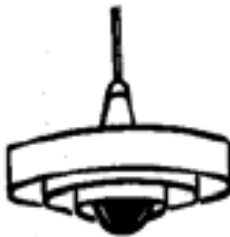
Concentric ring unit with incandescent silvered-bowl lamp
