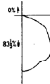
Porcelain-enameled ventilated standard dome with incandescent lamp
