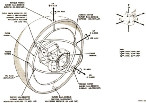
Figure 2.1-24. IMU Gimbal Assembly
